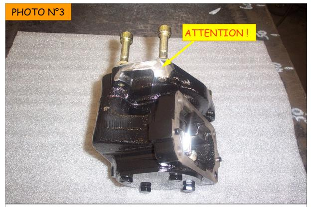
MAKE A LEVELLING ON THE PTO TO AVOIDE THE CONTACT WITH ANY PARTS OF THE ENGINE OF THE TRACTOR.
