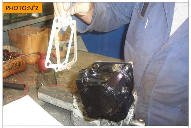
VIEW OF THE 3 GASKETS IN EQUIPMENT TO PUT BETWEEN THE PTO AND THE ENGINE.
