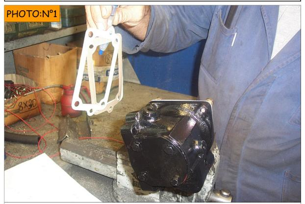
VIEW OF THE GASKETS IN EQUIPMENT TO PUT BETWEEN THE ENGINE AND THE PTO BASE.(LEAVE A LOOSE BETWEEN THE GEARS OF PTO AND ENGINE IF NECESSARY SUGGEST MIN. 0,50 mm MAX. 0,60 mm)
