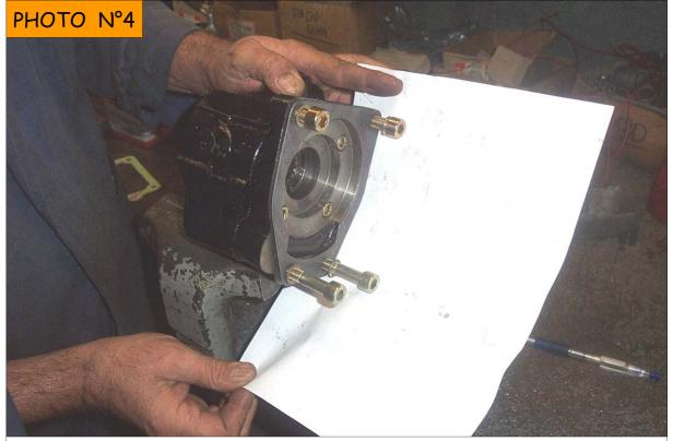
AFTER THE MOUNTING OF THE 3 GASKETS AND THE PTO WITH THE ENGINE GEARS BE SURE THAT BETWEEN THEM DO NOT EXIST ANY INTERFERENCES. AFTER THE MOUNTING OF THE PTO PUT A SHEET OF BLOCK-NOTES, IF IT PASS JUST ENOUGHT THE PTO WAS MOUNTED CORECTLY.
