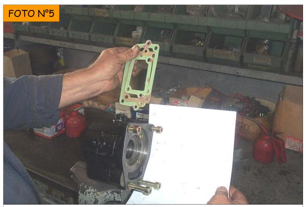
INTERPOSE THE THREE ENDOWMENT GASKETS BETWEEN THE MONOBLOCK AND THE PTO. AFTER FIXED THE PTO TO THE ENGINE VERIFY THAT A SHEET OF THE BLOCK NOTES GO THROUGH THE TWO CORPS. CHECK NO ONE CONTACT HAS TO BE. THEN THIGTEN WITH CAPACITY.
